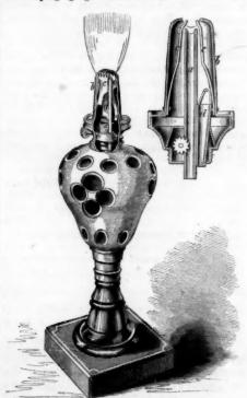
office of the plates, cc, is to conduct the heat from the flame downward into the currents of air, and to spread these currents into thin sheets in the proper position to bring them in contact with the ascending vapors of the oil.
